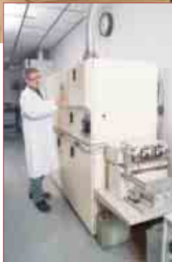
Lab Technician Keith Rozelle adjusts the Inductively Coupled Plasma (ICP) testing device. The device tests for wear metals in oil samples and is one of many new tests available in the refurbished laboratory facilities.
