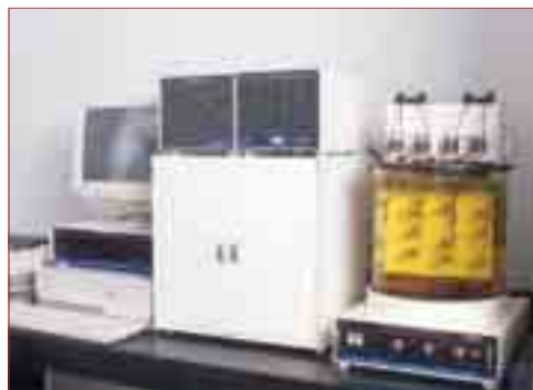
This constant temperature bath is used to determine the viscosity of test oils. This type of test may be run several times when comparing AMSOIL products with competitors' motor oils.
